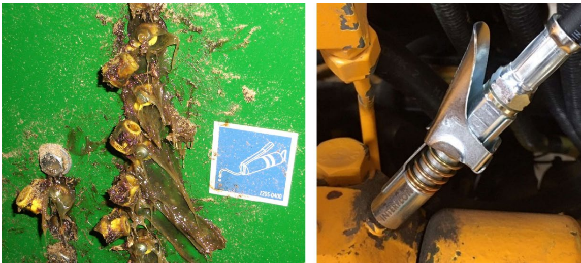
The Interflon G-Coupler keeps the grease nipple clean and ensures that the grease enters the nipple.
